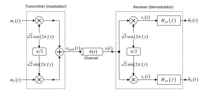
Figure 32: QAM Scheme
